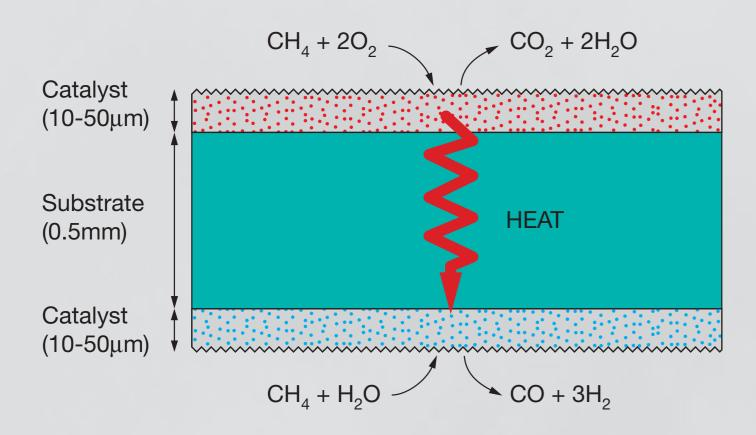
The principle of the Compact Reformer is to enhance heat transfer and catalyst activity using thin catalyst layers deposited either side of the compact heat exchanger.
