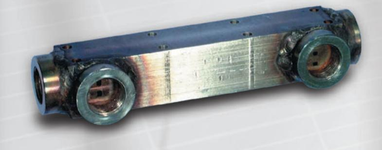
Proof-of-concept Compact Reformers, fabricated by diffusion bonding, have been successfully coated with catalysts and tested under realistic conditions, for extended periods. Extended tests over 500 hours have completed successfully.
